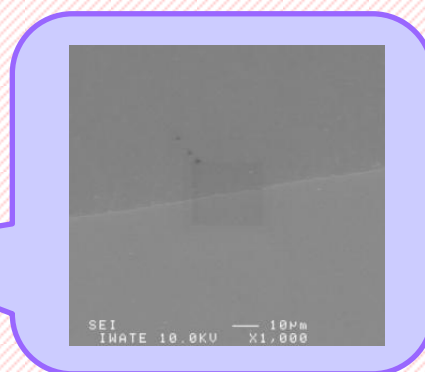
SEM photograph of bonding interface [× 1,000]
